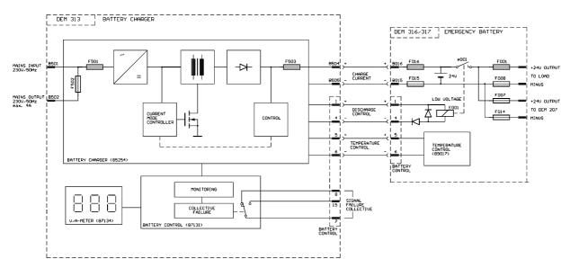
Fig. 1 Connection of the battery to the charging unit
